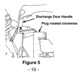
2. Since the plug is slightly wider than the discharge tunnel opening, rotate the plug clockwise slightly while inserting it (Fig. 5).
